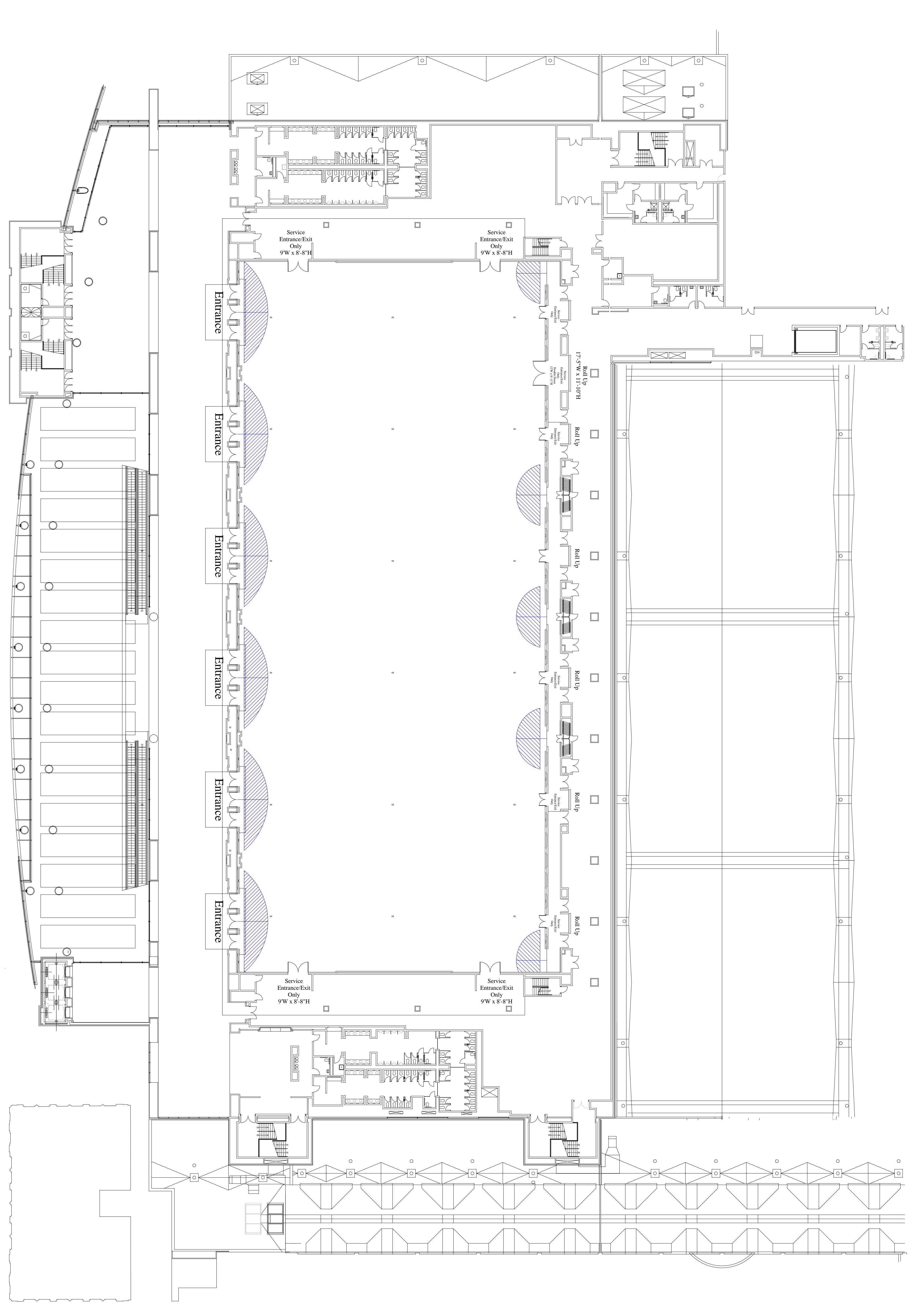
15' Clearance must be maintained in any direction from emergency exit doorways
