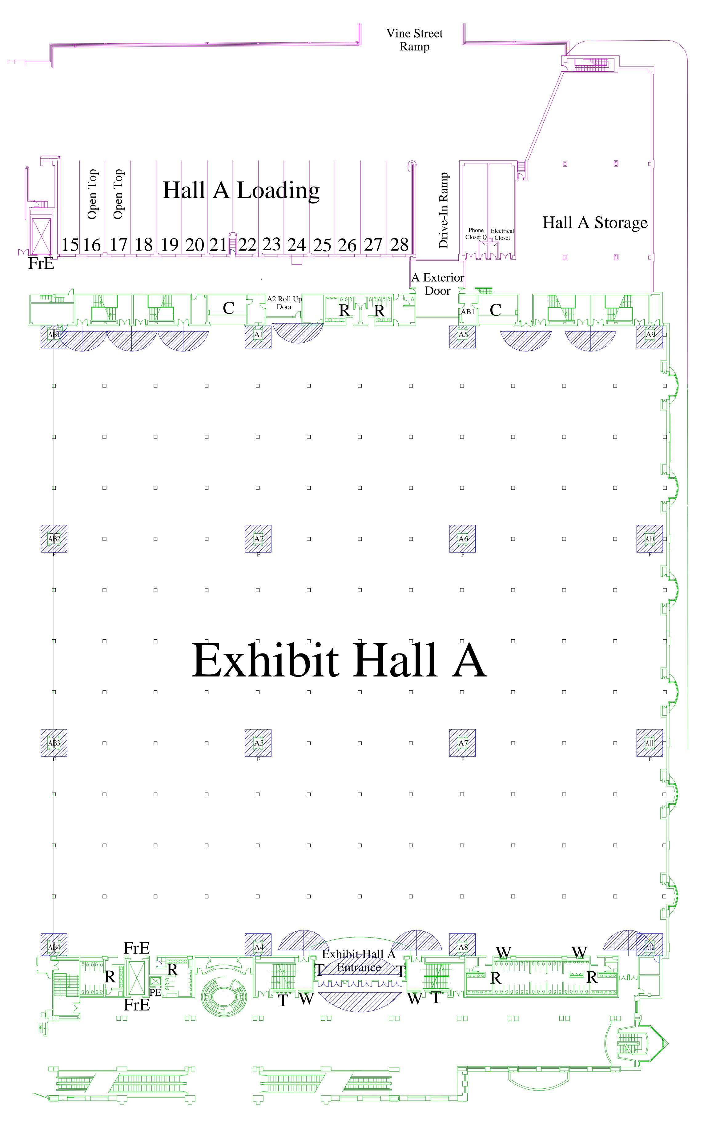
15' Clearance must be maintained in any direction from emergency exit doorways
