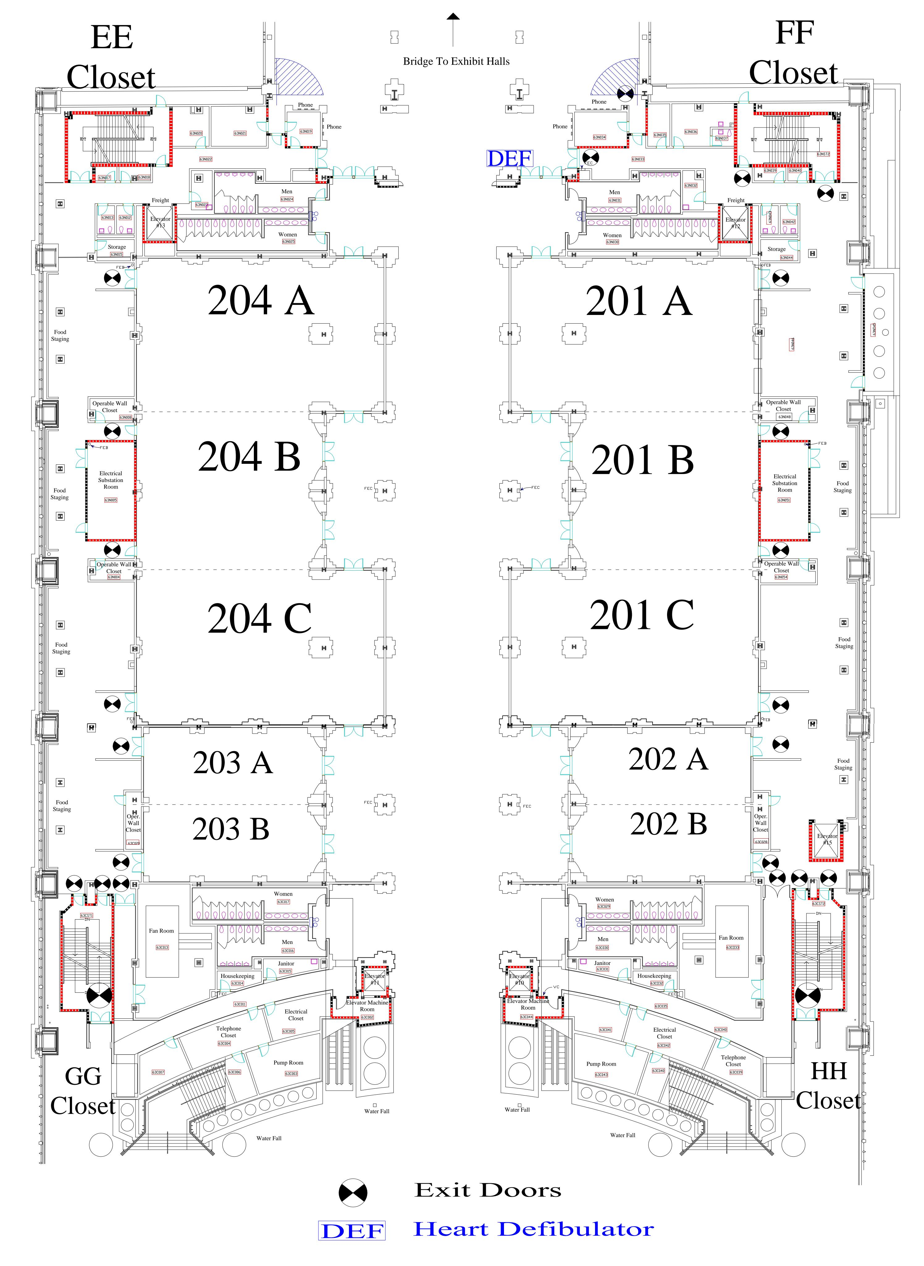
15' Clearance must be maintained in any direction from emergency exit doorways
