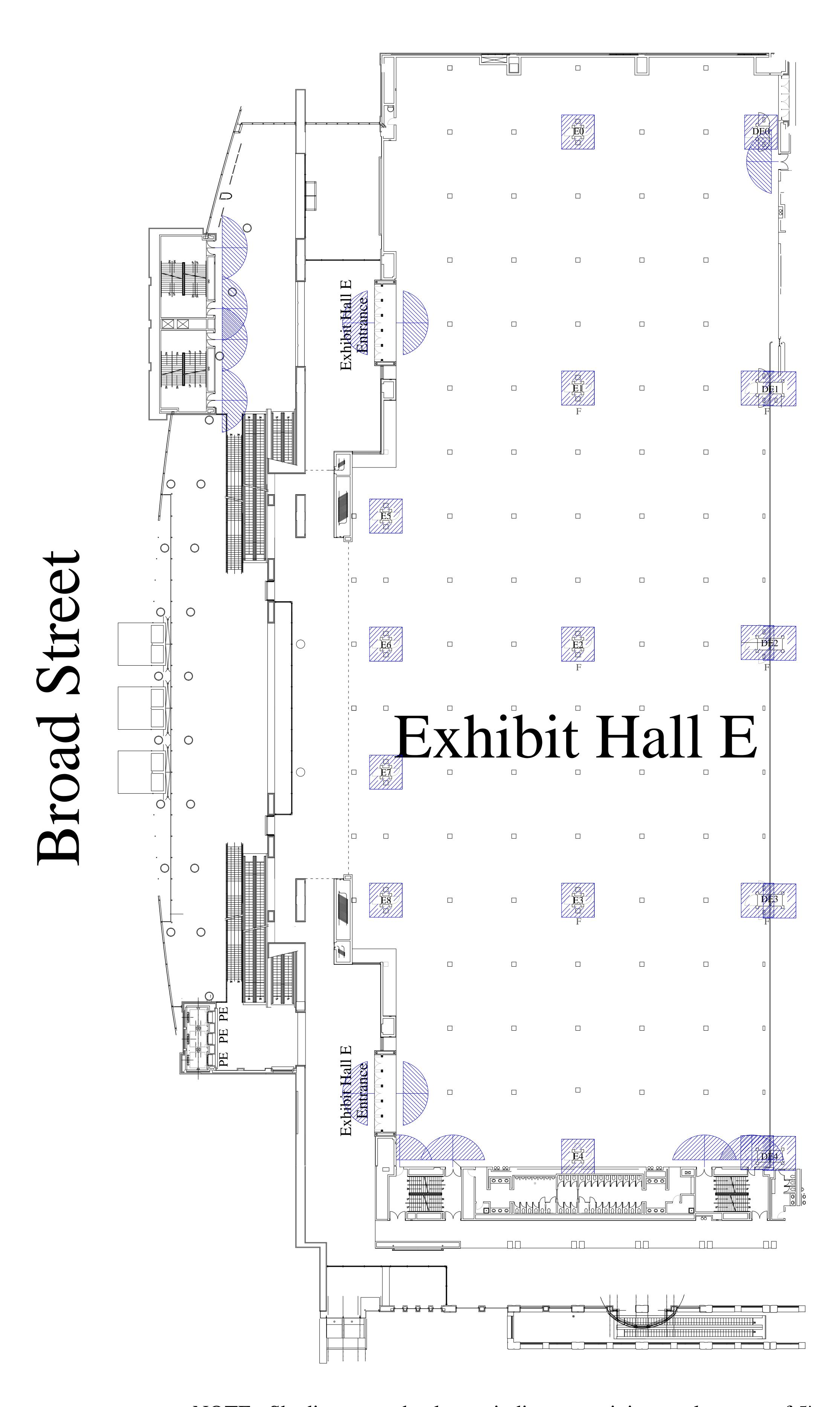
NOTE: Shading around columns indicates a minimum clearance of 5' on each side that must be maintained for access to electrical services and fire hose connections.
