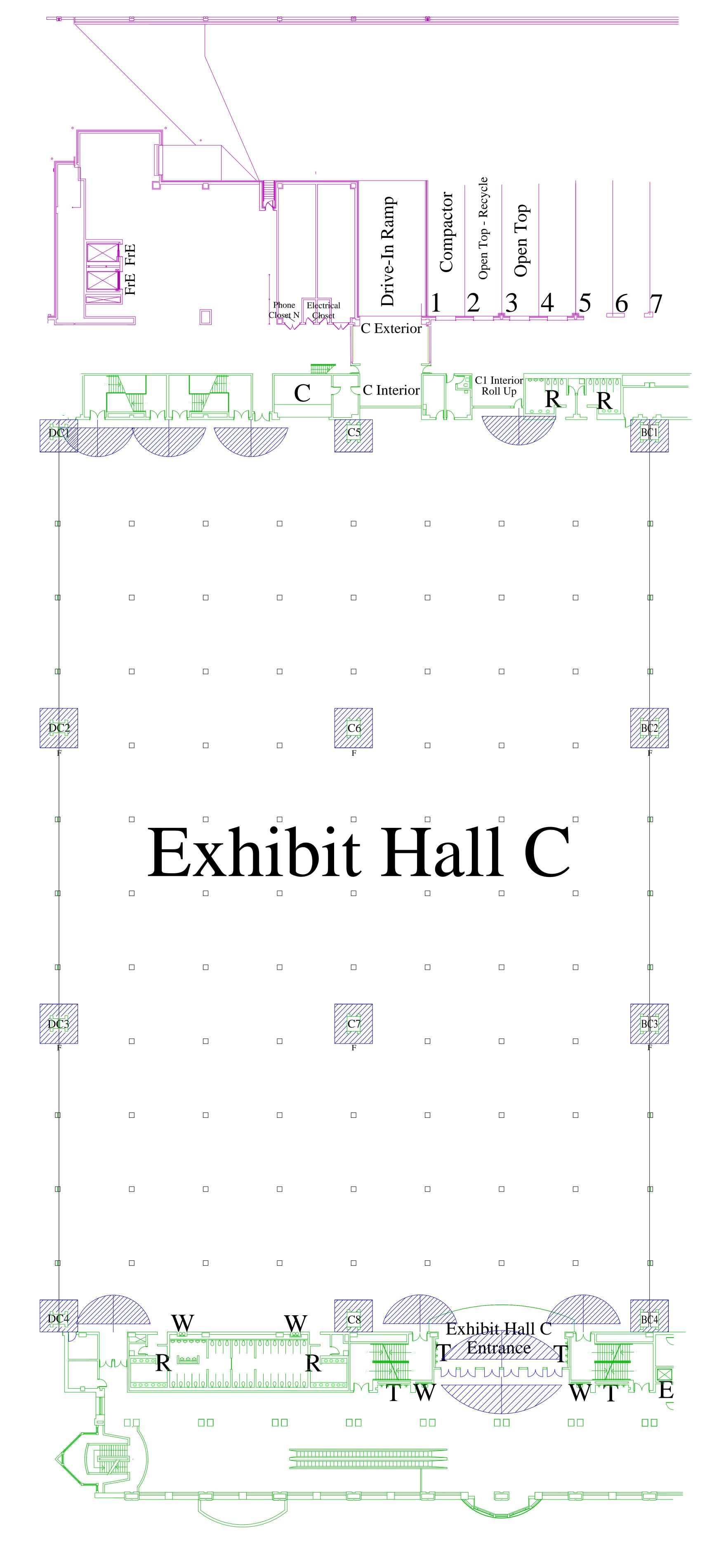
15' Clearance must be maintained in any direction from emergency exit doorways
