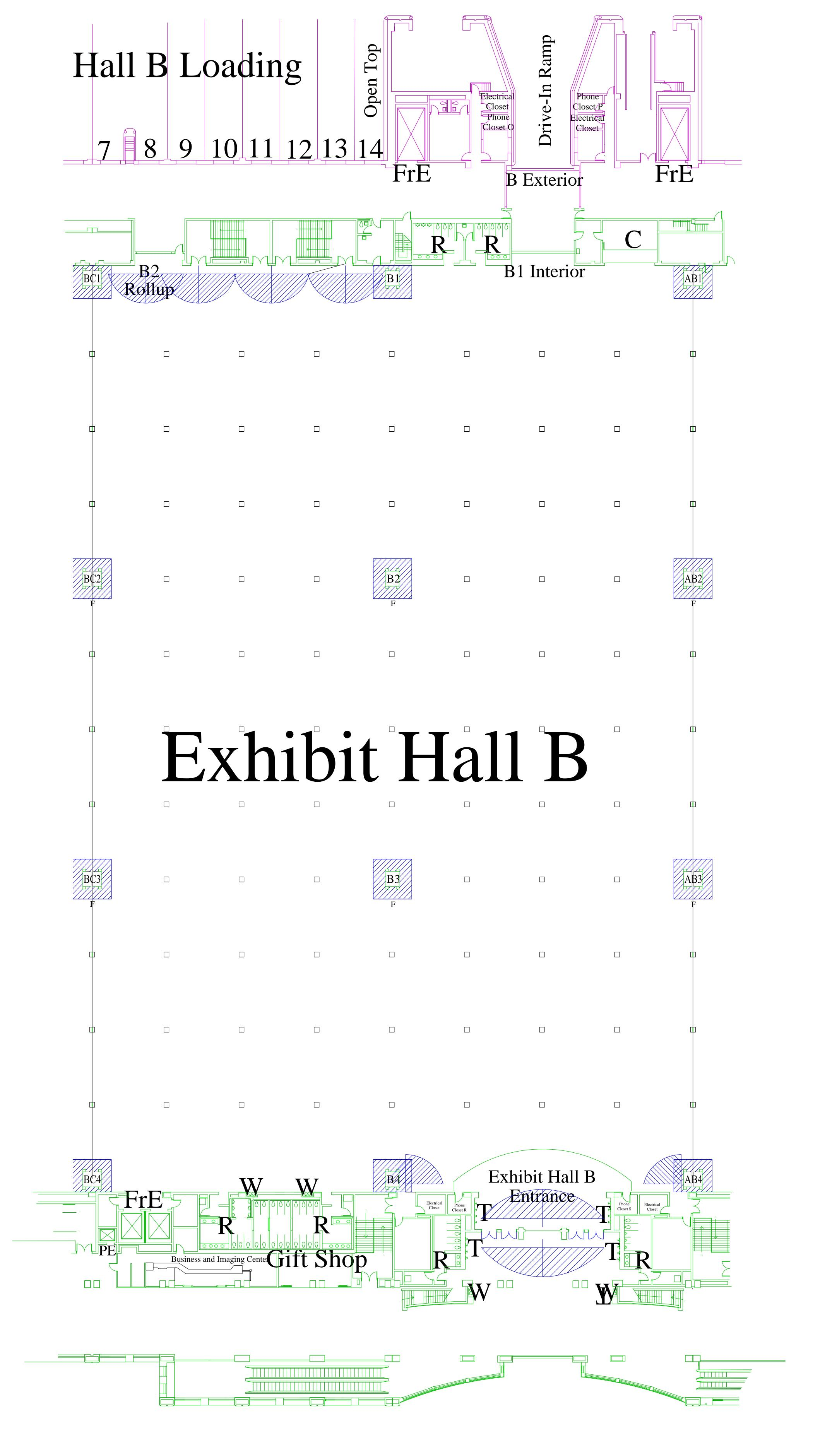
15' Clearance must be maintained in any direction from emergency exit doorways
